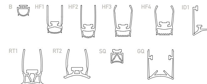
Self-extinguishing silicone seal (UL94-V0 certified).
